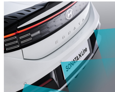
Rear Parking Sensors
